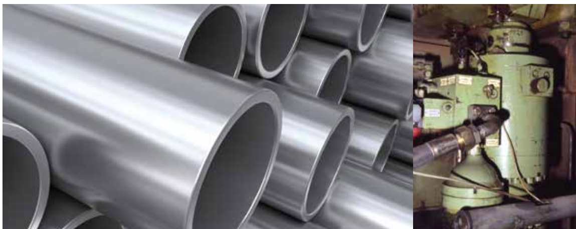
3 | Hydraulic cylinder on the continuous casting plant: oscillation at three hertz prevents the steel strand sticking to the inner wall of the ingot mould.
