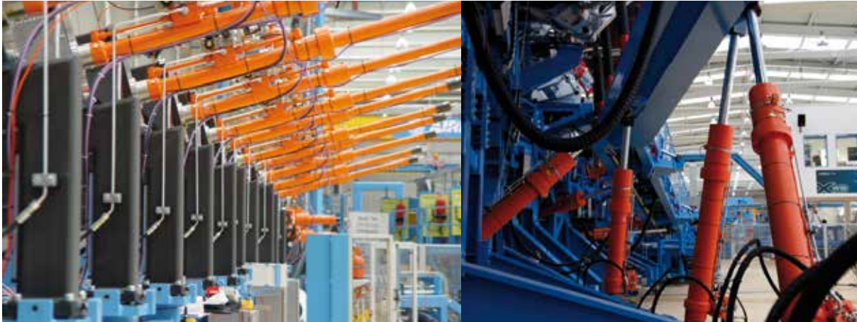
6 | Slat station with 14 hydraulic cylinders by Hänchen 7 | Hydraulic cylinder of the hexapod with flanged Ratio-Clamp®
