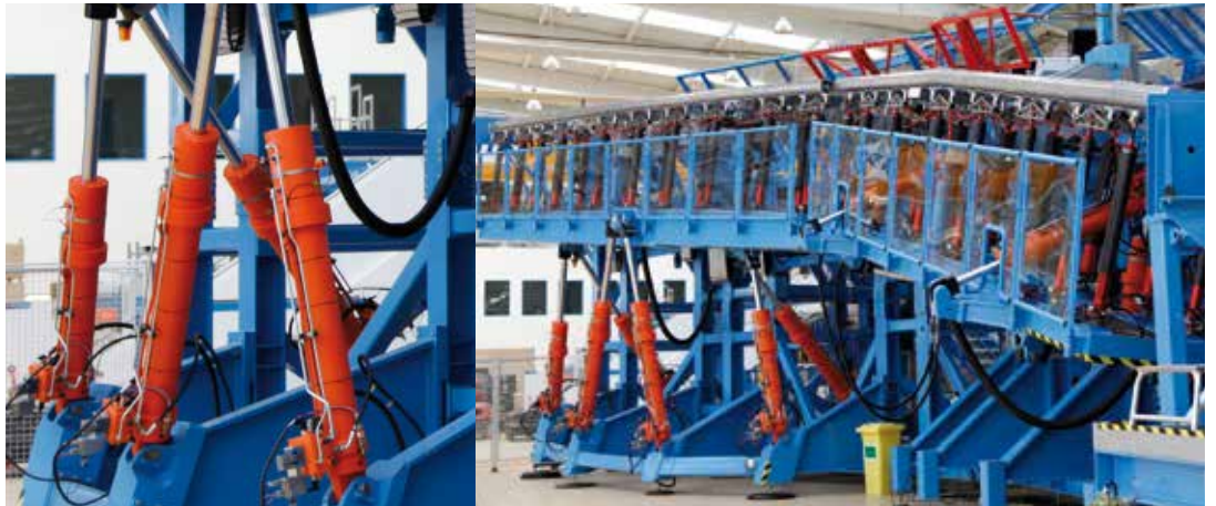
1 | Airplane wing test stand for simulating the airstream
