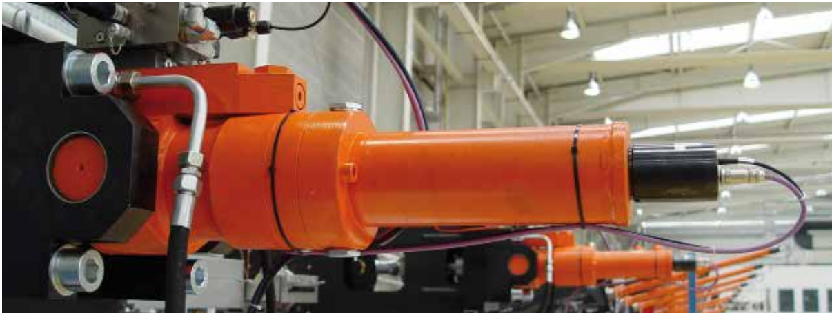
4| Hydraulic cylinder series 300 with position measuring system
