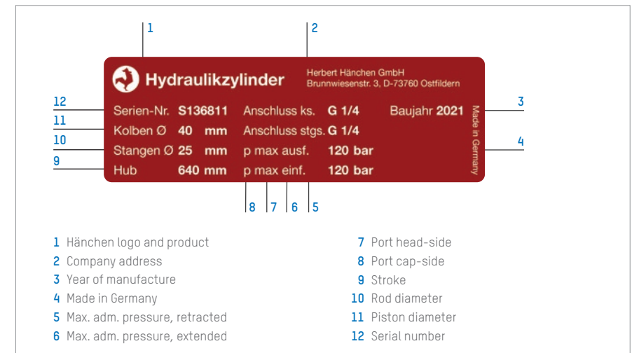
Figure 1: e.g. Type plate of hydraulic cylinder
